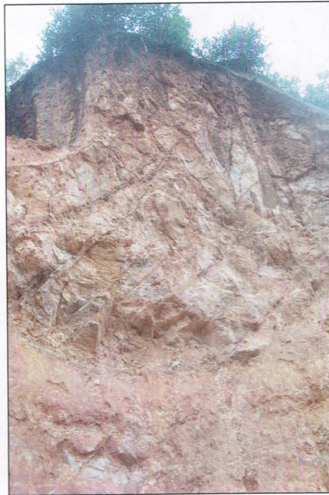
Photo 5: Head portion of the slide showing weathered Gneissic exposure with two sets of prominent joints.
